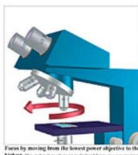
Focus by moving from the lowest power objective to the highest. This makes it much easier to find and focus on your specimen.
